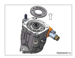
(18) Use grease in order to attach valve plate to the cover, following the pin.
